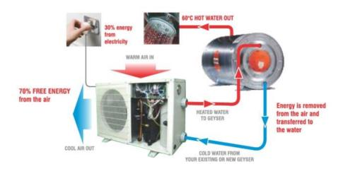
A heat pump works like an inverse air conditioner. It takes heat particles from the atmosphere, compresses them, pumps them into your geyser and circulates the water round.
